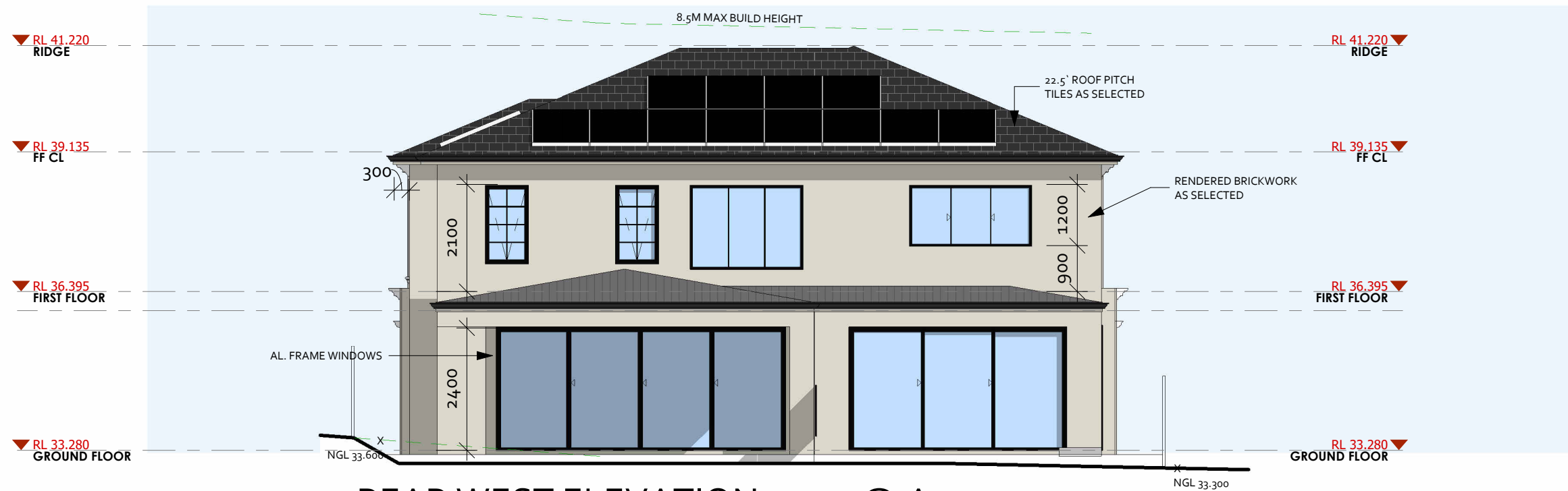
REAR WEST ELEVATION 1:100 @ A3
